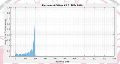
Figure 14 THD% in Voltage at the loading line in system 2 with loads from area-1
