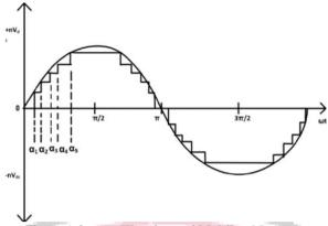
Figure 1 Output Waveform of Multilevel Inverter
