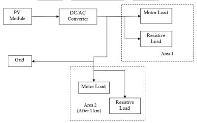
Figure 3 Proposed Hybrid energy system topology
