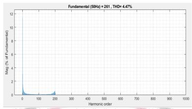
Figure 17 THD% in Current at the loading line in system 2 with loads from area-1
